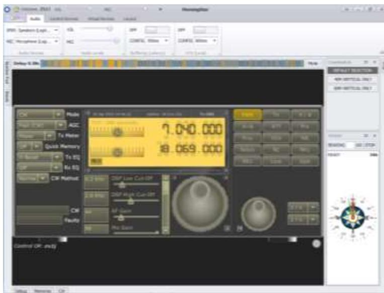
Many unnecessary buttons, sliders and dropdowns on the screen, not necessary for normal use, have been removed to make the screen less cluttered. Amongst those is the power slider that has been preset to 30 W to prevent the overdriving of the amplifier.
