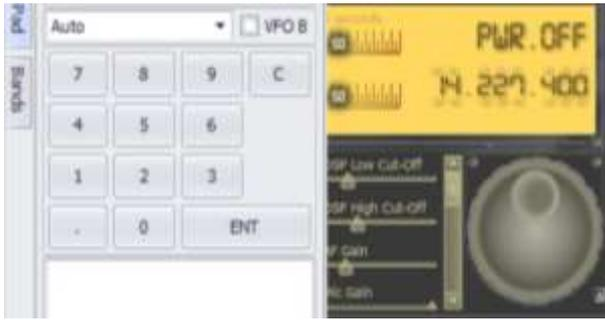
Using the number pad on the LH side of the virtual radio screen to type in the frequency,
