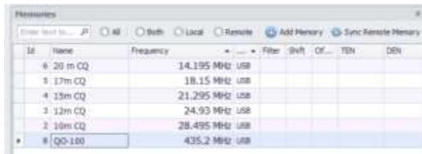
The relation between the 70 cm and the 3 cm downlink signal is linear and when you transmit on say 435.200 MHz the downlink signal will be on 10489.720 MHz which is displayed in the WebSDR as 10489720.00 kHz.
