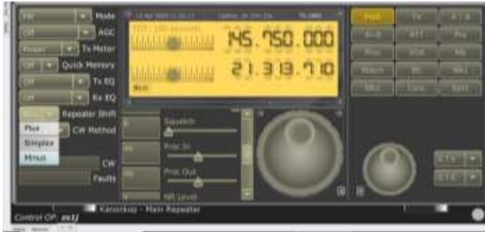
The Kanonkop repeater has already been added to the server memories. Click on the Memories tab at the LH bottom of the screen and then click on Sync Remote Memory to load.
