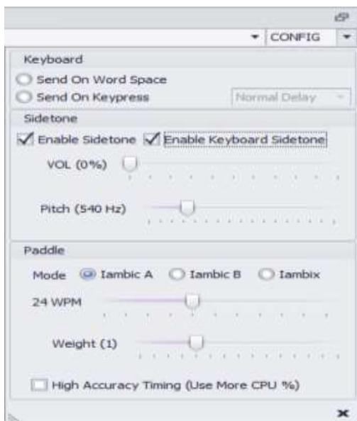
CW Config : Enable Sidetone and Enable Keyboard Sidetone boxes both ticked.
