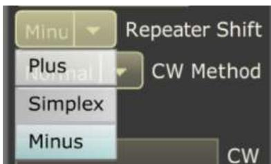
Repeater Shift enables the setup off simplex and repeater channels that can also be stored, edited and removed from Memories.
